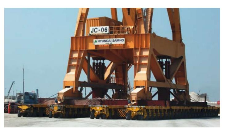
was a full 26m above ground level, to monitoring the wind speed and constantly maintaining the crucial stability angle of 6.90°. It is a great testimony to the highly motivated teamwork between the professionals of AJHL and its client that the project was executed so smoothly.
